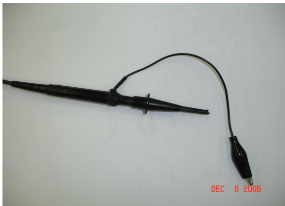
FIG. 4: Photograph of an oscilloscope probe that significantly changed the frequency of the reference pitch oscillator when connected to the theremin.
