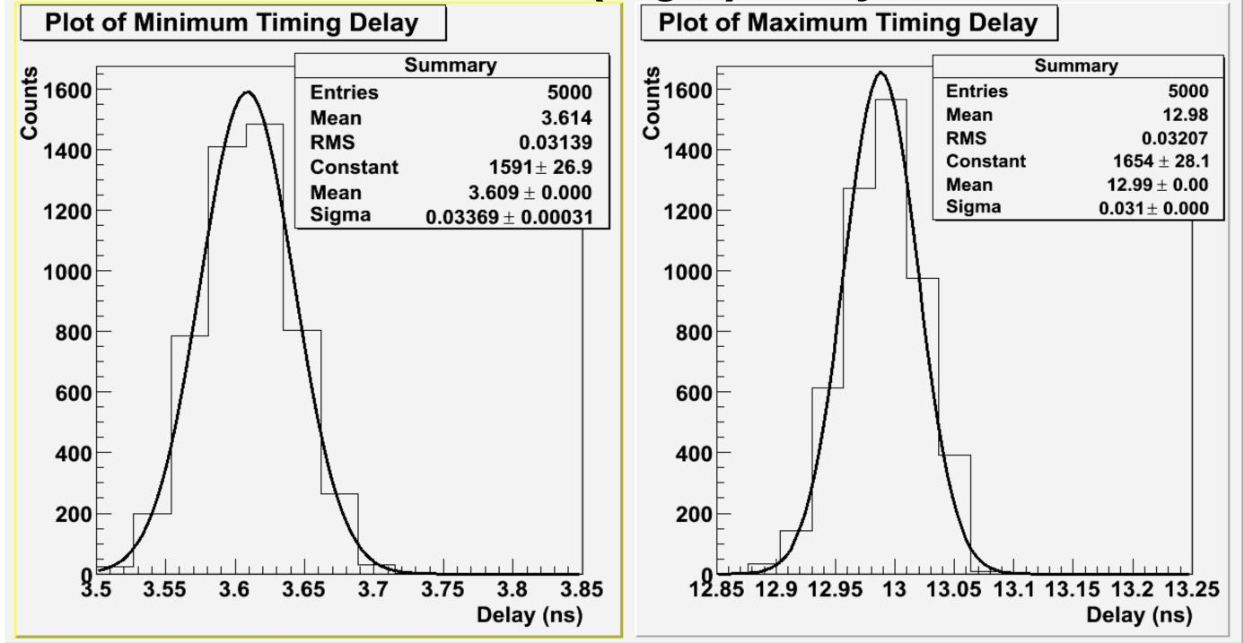
Measurements of the timing delay were taken with the previous standard electronics used in high energy physics, the CAMAC system. The measurements show **~30ps of noise**. *Get more information about: STAR at*
