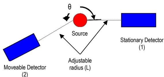
**Figure 1: Apparatus used for angular correlation measurements. Detectors consist of a scintillator with a photomultiplier tube. Each PMT was operated at 1600V.**
