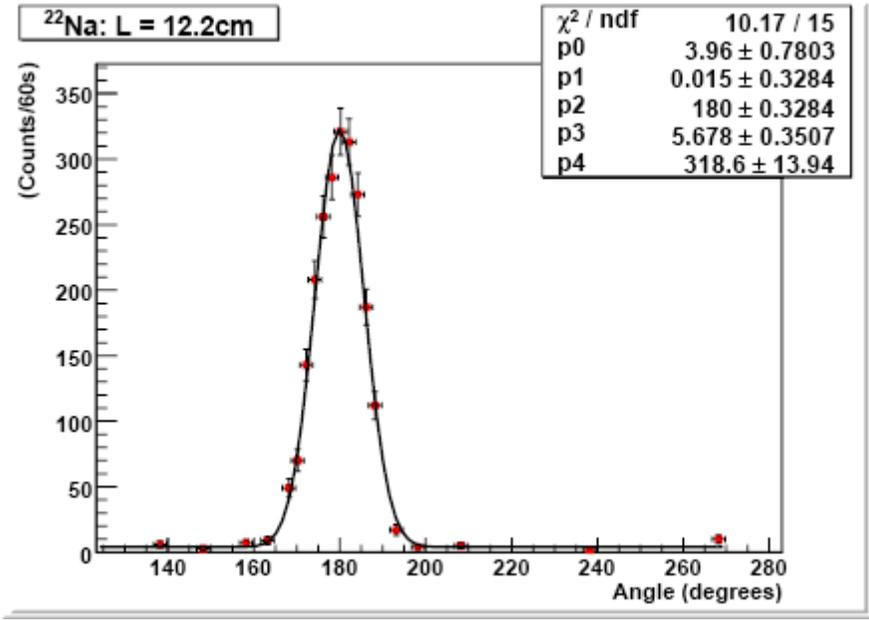
Figure 6: Plot of  $^{22}\text{Na}$  data with  $L = 12.2\text{cm}$  fit to gaussian. Fit equation:  $319e^{-\frac{1}{2}\left(\frac{\theta-180}{5.68}\right)^2} + 4.0$
