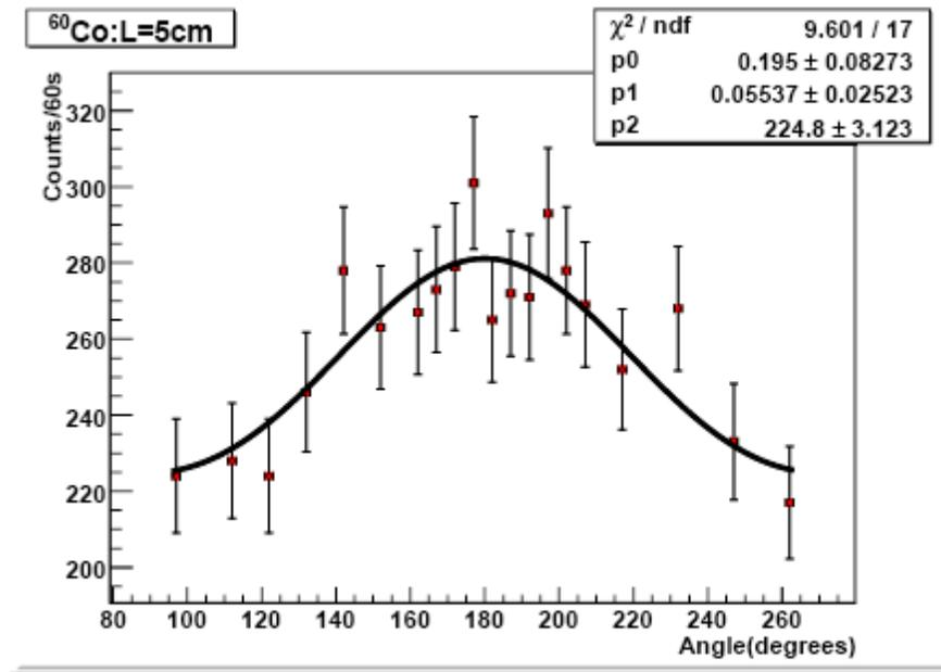
Figure 7: Plot of  $^{60}\text{Co}$  data with  $L = 5\text{cm}$ . Fit equation:  $224.8(1+0.195(\cos\theta)^2+0.055(\cos\theta)^4)$
