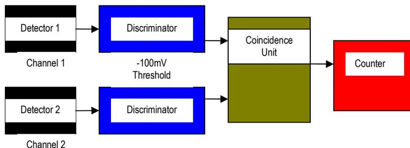
**Figure 3: Experimental setup used to make angular correlation measurements.**
