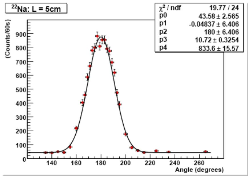
Figure 5: Plot of  $^{22}\text{Na}$  data with  $L = 5\text{cm}$  fit to gaussian. Fit equation:  $834e^{-\frac{1}{2}\left(\frac{\theta-180}{10.72}\right)^2} + 43.6$
