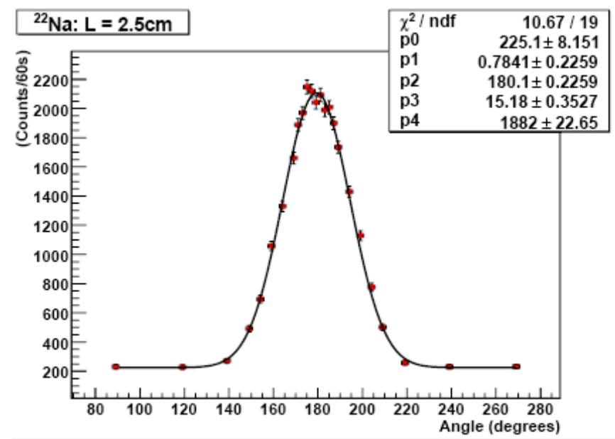
Figure 4: Plot of  $^{22}\text{Na}$  data with L = 2.5 cm fit to gaussian. Fit equation:  $1882e^{-\frac{1}{2}\left(\frac{\theta-180.1}{15.18}\right)^2} + 225.1$
